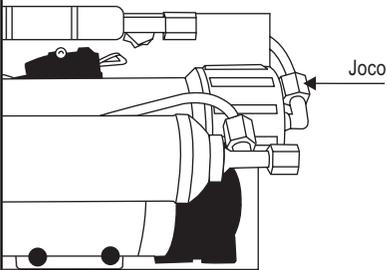
5 Remove the membrane housing cap anticlockwise.
