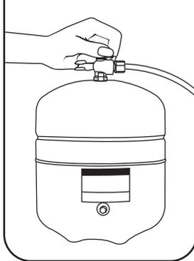
4 Loose the Joco fitting anticlockwise.
