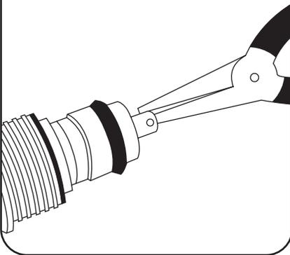
7 Install the membrane by carefully pushing the spigot end into the socket at the far end of the housing until completely in.
