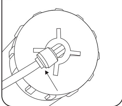
4 Remove the membrane housing cap anticlockwise.
