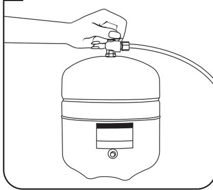
3 Loose the Joco fitting anticlockwise.
