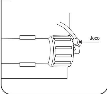
4 Remove the membrane housing cap anticlockwise.
